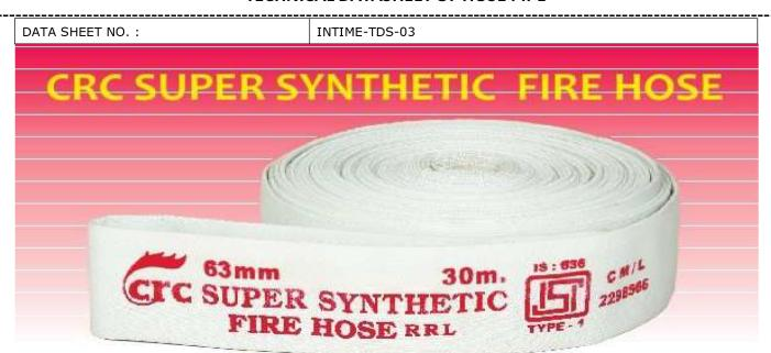
**CRC Super Synthetic fire Hose** is made out of High Tenacity Synthetic Yarn to ensure fool proof performance The lining is seamless type of EPDM rubber compound for excellent protection against ageing and tackiness. The Synthetic jacket of the hose is completely inert againt attack from middle and fungus. Moreover, being a 100% synthetic it can be dried very easily o form small and compact rolls which can stored and moved around easily.
