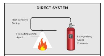
In the Direct system, heat-sensitive tubing also acts as an extinguishing agent delivery system. When a fire is detected, the tube bursts at that point, forming a miniature nozzle that sprays the extinguishing agent. Ideal for places where fires can break out in localized areas.
