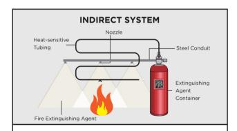
In the Indirect system, heat-sensitive tubing only acts as a detection device. In the event of a fire, the extinguishing agent is delivered through a steel pipe and sprayed across the entire area through strategically placed nozzles. Ideal for areas where fires can break at multiple points.
