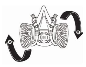
Turn adapter ¼ turn clockwise to stop. To remove adapter, turn ¼ turn counter-clockwise.
