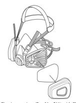
Place filter into retainer (Part No. 501) with filter printing facing towards the 603 adapter. Snap together and ensure the filter seal is free from creases or gaps.
