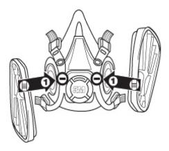
Align notch on edge of  $60\overline{3}$  adapter with facepiece mark, as shown, and push together.
