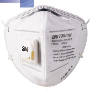
The 9504IN & 9504INV are at least 94% efficient against fine dusts, water & oil based and non-volatile liquid aerosols down to 0.1 micron. Its Penetration is lower than 6% and pressure drop is lower than 21 mm of  $H_2O$ .
