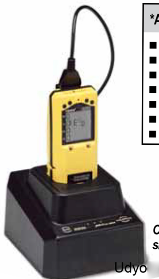
M40 Multi-Gas Monitor shown with optional SP40 Sampling Pump attached
