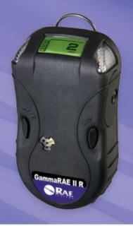
The RAE Systems GammaRAE II R is a rapid gamma radiation detector and dosimeter in a single instrument. The GammaRAE II R is designed specifically to meet the needs of national security and emergency responders. Due to its high sensitivity at low radiation levels, GammaRAE II R can alert users of the presence of a radiation threat well before reaching health-threatening levels. Its high range and dosimeter functionality allow security and emergency responders to track their dose.
